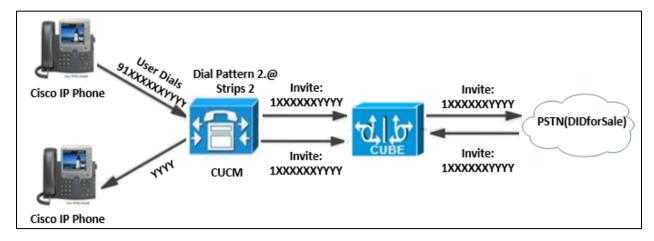
Figure 6: PBX to PBX via DIDforSale Call
