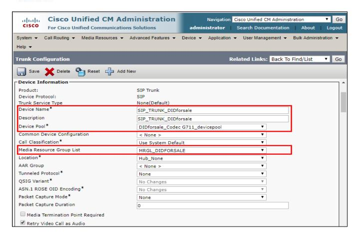
Figure 13: SIP Trunk to Cisco UBE
