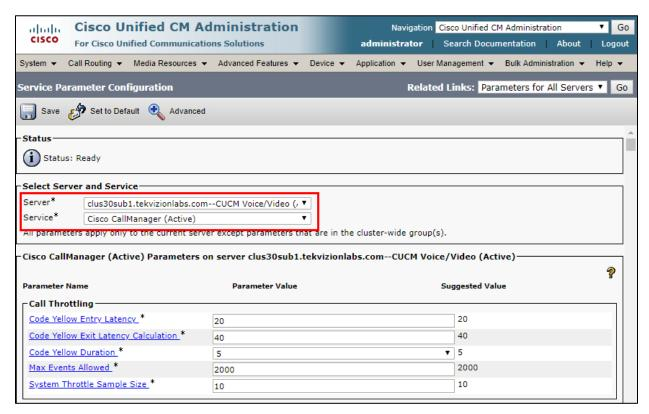
Figure 8: Service Parameters
