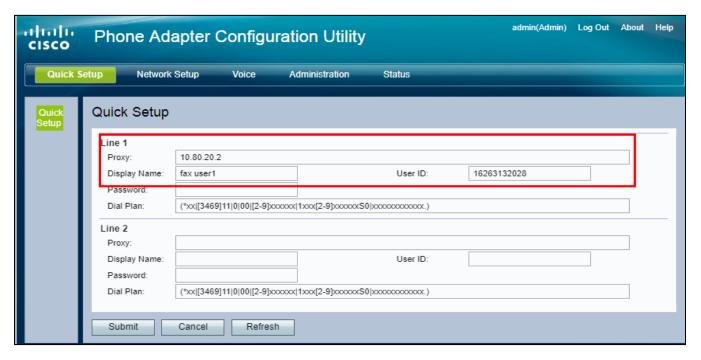
Figure 21: FAX ATA Configuration
