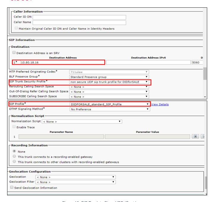
Figure 15: SIP Trunk to Cisco UBE (Cont.)
